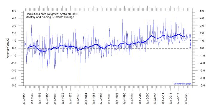
Diagram showing area weighted Arctic (70-90°N) monthly surface air temperature anomalies (<u>HadCRUT4</u>) since January 1957, in relation to the WMO <u>normal period</u> 1961-1990. The thin line shows the monthly temperature anomaly, while the thicker line shows the running 37-month (c. 3 year) average.
