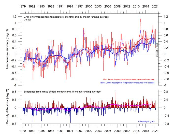
Global monthly average lower troposphere temperature since 1979 measured over land and oceans, respectively, according to <u>University of Alabama</u> at Huntsville, USA. Thick lines are the simple running 37-month average, nearly corresponding to a running 3-year average. Reference period 1981-2010.
