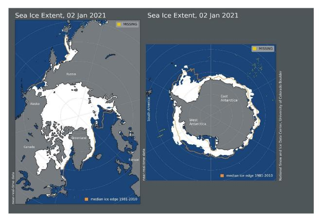
Sea ice extent 2 January 2021. The median limit of sea ice (orange line) is defined as 15% sea ice cover, according to the average of satellite observations 1981-2010 (both years included). Sea ice may therefore well be encountered outside and open water areas inside the limit shown in the diagrams above. Map source: National Snow and Ice Data Center (NSIDC).
