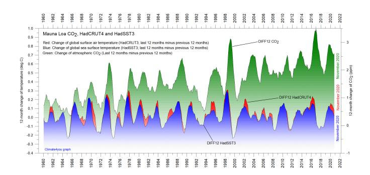
12-month change of global atmospheric  $CO_2$  concentration (<u>Mauna Loa</u>; green), global sea surface temperature (<u>HadSST3</u>; blue) and global surface air temperature (<u>HadCRUT4</u>; red dotted). All graphs are showing monthly values of DIFF12, the difference between the average of the last 12 month and the average for the previous 12 months for each data series.
